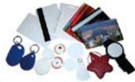
RFID tags come in a wide variety of shapes and sizes: Plastic/paper Card, Key Fobs, ABS/PVC Tag, clear tag, etc. assist to expand more applications.
