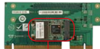
Wireless module on the PCI/ PCIe mini card inside IBX POS PC
